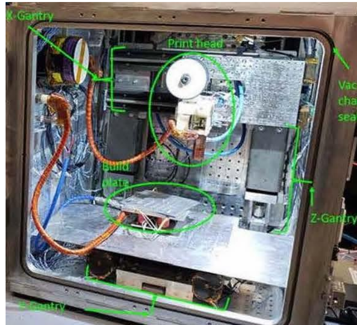
Made in space “Vulcan” – integrates Additive manufacturing and CNC machining
