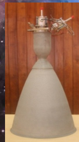
LUPEX Mission: High Thrust 3.1kN and 1.5kN Throtttable Engines
